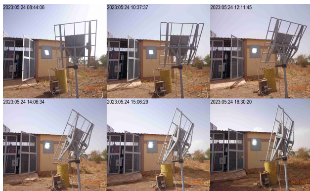
Figure 14: Sequence of images of the focal spot during the solar tracking test done on May 24 th , 2023
