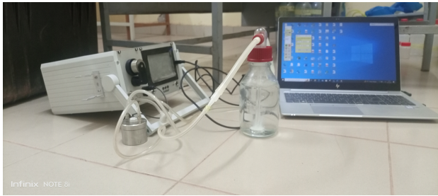
Figure 2: Experimental set-up for the measurement of radon in water.
